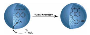
A general method for preparing site-isolated polymeric catalysts is presented. Linear chloromethyl and azide polymers have been sequestered within polyurea microcapsules and small molecule catalysts soaked through the shell walls to functionalize the soluble polymers. Reaction onto each type of support is quantitative and MacMillan, DMAP, and TEMPO test catalysts are shown to have faster reaction rates than the analogous resin-supported catalysts.
